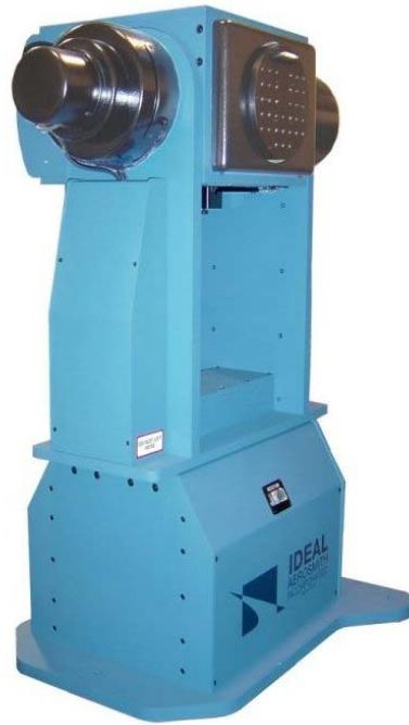
torque motors, precision optical encoders, and the Ideal Aerosmith AERO 832 microprocessor-based three-axis motion controller. Positions, rates, and accelerations are commanded locally from the front panel keypad or remotely through the standard IEEE-488 and RS-232 computer interface. This test table system is designed for ease of operation and is programmed with the Ideal Aerosmith Table Language (ATL) for remote operation.
