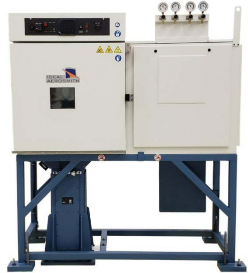
1291BLX temperature chamber with 18 inch tabletop in vertical axis configuration
