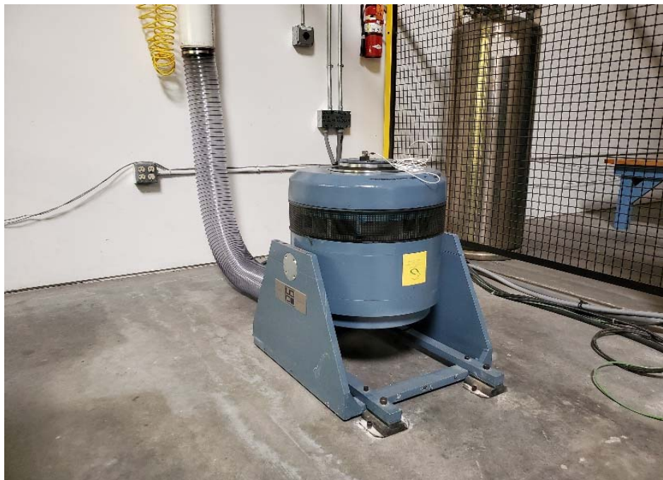
Figure 2 Model Unholtz-Dickie S092 Linear Shaker at the Inertial Test Lab
