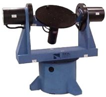
Model 1533 Three-Axis Rate and Positioning System
