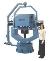
reliable motion control. The table can be operated from the AERO Controller front panel for local control or through a computer interface for remote control.
