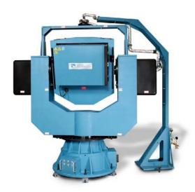
rotation based on specific customer requirements. For limited rotation applications, these tables have wire wrap allowance that provides a cost effective alternative to slip rings. Wire wrap test tables are designed for high reliability, minimal electrical noise, and low maintenance.
