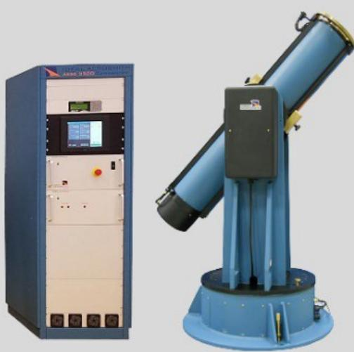
The Ideal Aerosmith Trip Guardian™ 2203-TH-NM Automated Three-Axis, Non-Magnetic Positioning Table System is intended for use in calibration and verification of MWD downhole directional instruments, including magnetometers, gyroscopes, and accelerometers.
