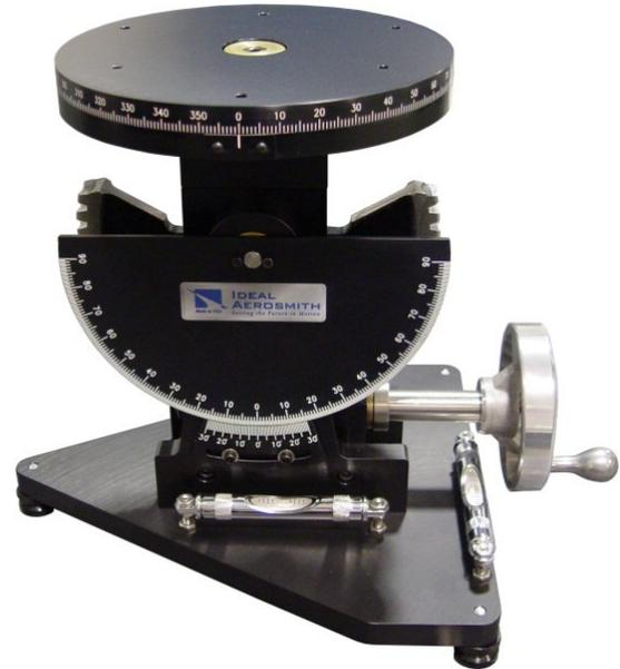
increments are optional. A spring-loaded steel ball engages detents in the bottom of the table top, locking it into position for quick setup. The detents are located every 45°. Tables with optional engraved marks every 1° have detents every 15°. The tension is adjustable for the positioning detents on the table top.
