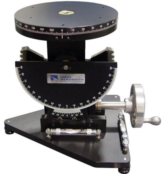
increments are optional. A spring-loaded steel ball engages detents in the bottom of the table top, locking it into position for quick setup. The detents are located every 45°. Tables with optional engraved marks every 1° have detents every 15°. The tension is adjustable for the positioning detents on the table top.
