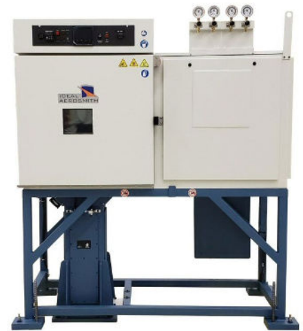
1291BL temperature chamber with 18 inch table top in vertical axis configuration
